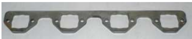
EX11 - Header flange for 472/500cid Cadillac. For use with 1.75" or 1.875" tubing, 3/8" steel.
